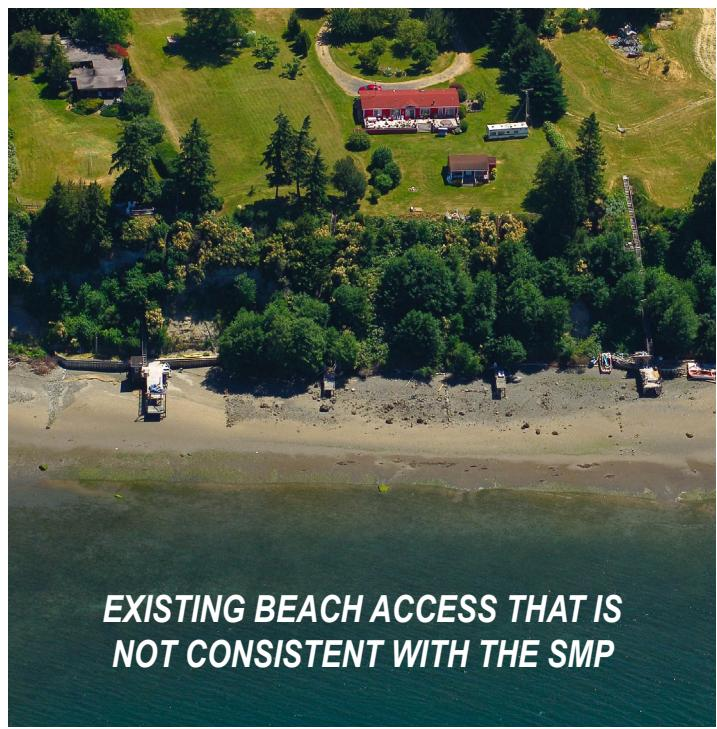
This reach of Holmes Harbor includes several homes with separate beach access structures, all of which have landings that include overwater structures, and in some places hard armoring with fill. The SMP encourages joint use beach access structures, and requires that landings must be landward of the OHWM (or if this is not feasible, limited to 25 square feet on piles).
