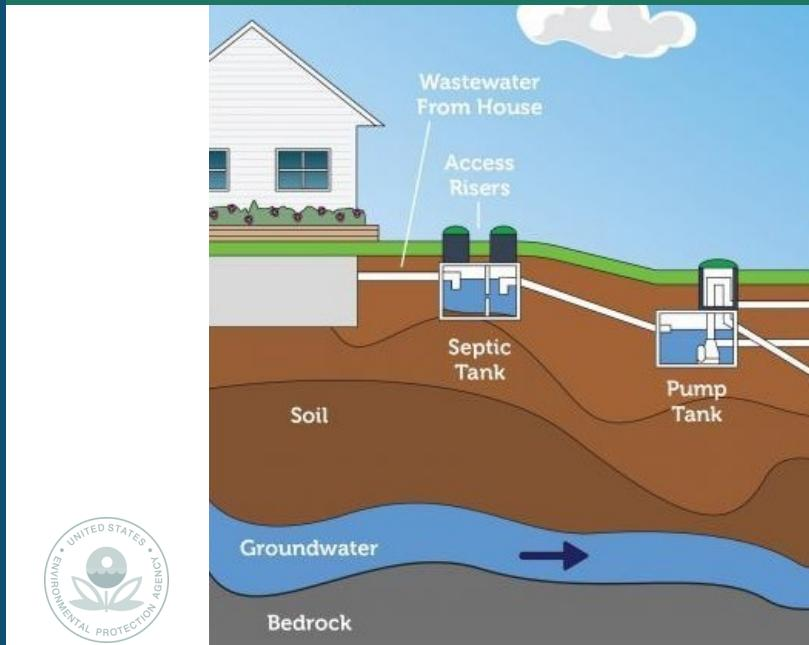
Consisting of a septic tank, pump tank, pump, and drainfield, these types of systems utilize pressure to move wastewater throughout the system. The pump tank is similar to a septic tank in size, and houses a pump and different alarm floats. These systems typically are timer set so the pump doses the drainfield, evenly distributing a set amount of the wastewater to the lines at various times of the day. Pumps, alarms, and panels require electrical hookups and wiring that can also malfunction.
