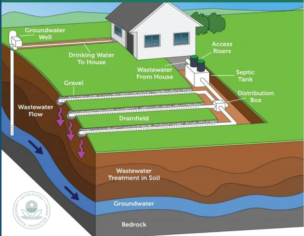
A sub-surface system of perforated piping organized into trenches or a bed, drainfields receive wastewater that has been treated by the septic tank and piped equally through the distribution box. Wastewater then exits the drainfield through one of several small openings to the soil below which contains microbes that will continue treatment. Unlike other drainfields with more complex components, conventional systems use gravity to move the wastewater throughout the system.
